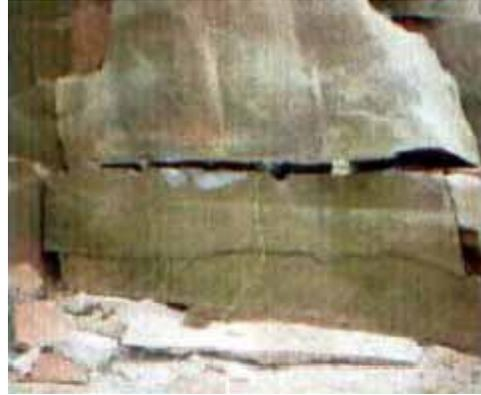
CARDOX Tubes applied horizontally to lift a block along its natural bed plane.
