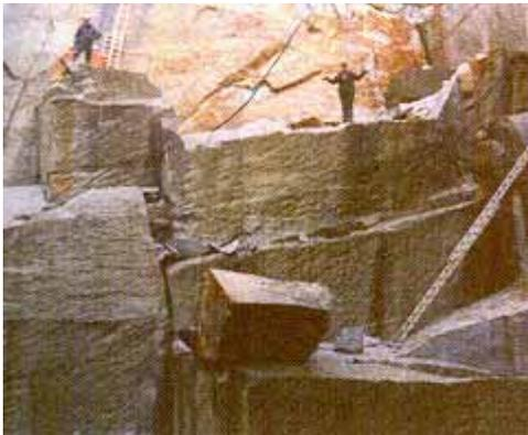
When using CARDOX, very little wastage results, as the gas splits and heaves along natural fissures and bed planes.
